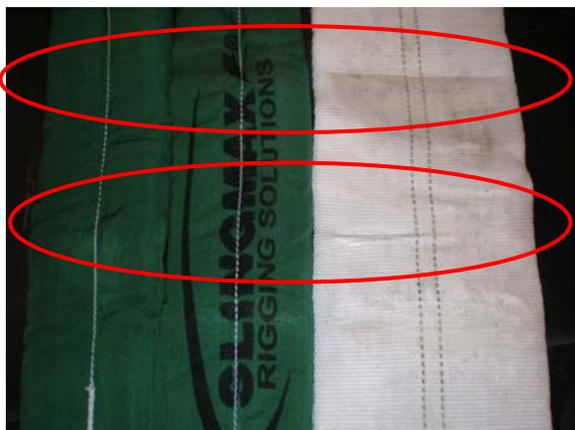
No damage was found on the Cornermax<sup>®</sup>/Dyneema<sup>®</sup> Sleeve after this test.
