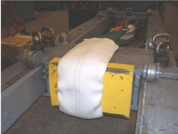
The 10" Cornermax<sup>®</sup>/Dyneema<sup>®</sup> Sleeve was placed over a TPXC 15,000 and pulled over the 90° edges of a sharpened steel plate.
